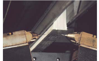
Nozzle blockages caused by degradation of the adhesive in the melt tank is a common problem with standard hot melts – eliminated when using BAMFutura hot melts because of the resistance to oxidation built into the product.
